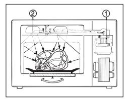
In a microwave oven there is a high-frequency tube called a magnetron ①. This converts electrical energy into microwaves. These microwaves are distributed evenly throughout the oven interior by a metal fan blade known as a stirrer ② -, rebounding off the metal sides of the oven interior and thereby reaching the food from all sides. Microwave distribution is improved by engaging the turntable.
